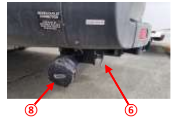
Separate BLACK and GREY water outlets
