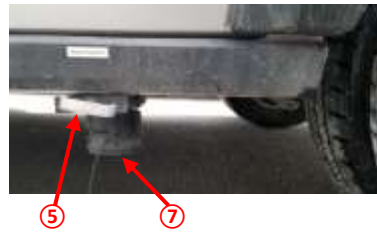
Separate BLACK and GREY water outlets
